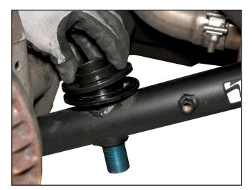
9. Install upper spring isolator on spring.
