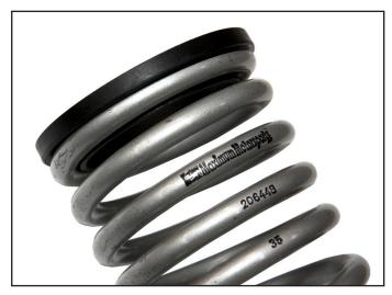
10. Install the spring onto the control arm. Make sure the spring's pigtail is pointing toward the driver side of the car. Note that both rear springs are identical, and the spring's pigtail is oriented the same (pointing toward the driver side of the car) for both rear springs.
