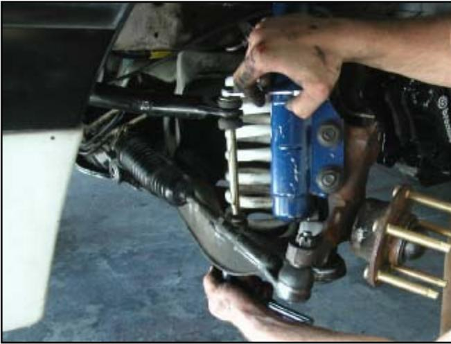
17. Turn the spindle to its maximum toe-in position. Place a floor jack under the control arm near the ball joint. Leave about ½" of clearance between the floor jack and the control arm.
