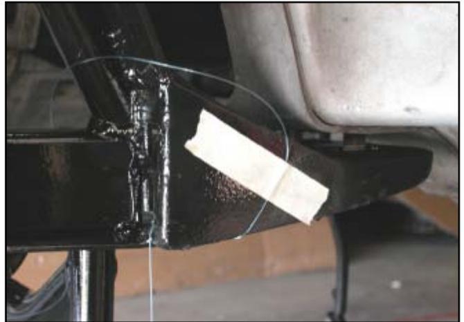
52. Stick pieces of masking tape to the ground directly under the tip of each plumb bob.
