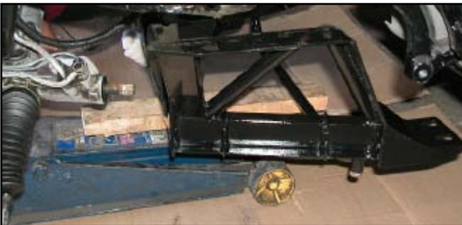
42. Slowly raise the K-member into position underneath the front of the vehicle. Check to make sure that nothing is getting pinched as you raise the K-member. There may be brake line interference on one or both sides of the car. The lines may be carefully bent as needed, to provide required clearance. If necessary, trim the plastic fender liner.
