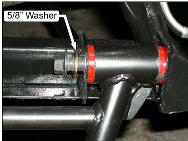
81. Thread a factory nut onto each pivot bolt.
