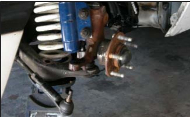
22. Strike the spindle just below the strut, where the ball joint attaches to the spindle, with a large hammer. Do this until the ball joint taper comes free from the spindle.
