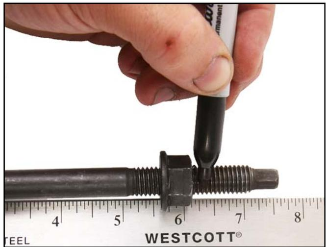
88. Use a hack saw or grinder to cut each bolt at the mark placed in Step 87.
