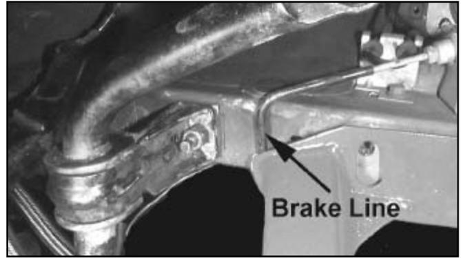
43. Once the K-member is within 1/2" of the frame rails, stop and install all eight bolts that hold the K-member to the chassis. Note that each of the two pairs of rearward bolts thread into nuts captured by a single removable nut plate.
