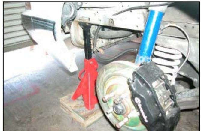
5. Level the car by measuring from the bottom of the rocker panels to the ground. Adjust the height of the jackstands to get the car as level as possible.
