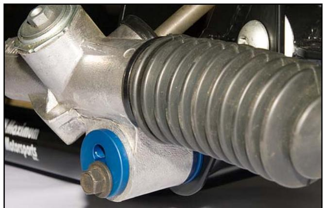
93. Check the orientation of the clamps which secure the rubber rack bellows boots to the rack housing. If the clamp bolt is installed towards the K-member as shown below, the clamp bolt may prevent the steering rack from being fully seated against the K-member. If necessary, rotate the position of the boot clamps.
