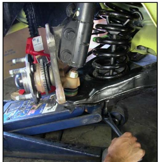
24. Raise the control arm 1/2" with the floor jack. Remove the ball joint nut completely.
