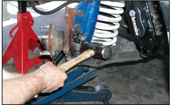
23. For cars equipped with conventional front coil springs, use an internally mounted coil spring compressor and compress the front coil spring. Most auto part and equipment rental stores rent this type of spring compressor.
