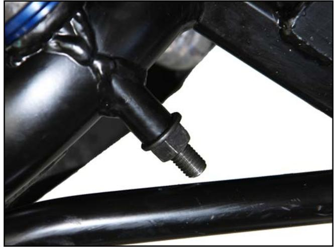
92. Snug the factory nuts onto the steering rack bolts. With offset steering rack bushings, ensure that the bushings as well as the spacers behind the rack are oriented correctly. The three holes in each bushing should be in a vertical line with the center of the bushing.
