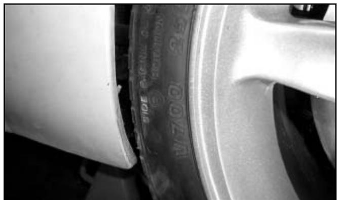
**AFTER TRIMMING THE FENDER EXTENSION**
