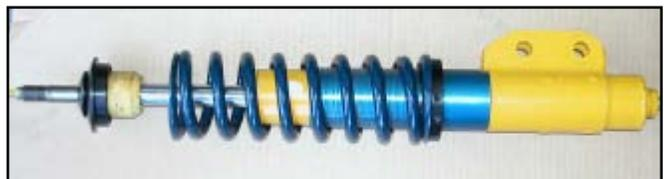
102. Install the coil-over strut assembly into place in the caster/camber plate. Adjust the spacers between the upper spring perch and the caster/camber plate as per the MM Front Coil-over Kit instructions to allow for maximum bump travel.
