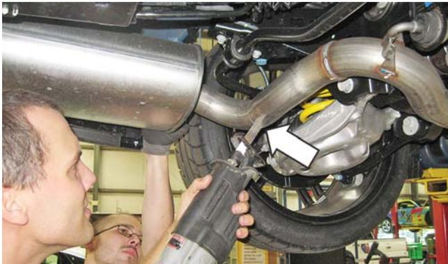
3. With the pipe cut; slide the hanger out of the rubber mount and remove the muffler assembly from the vehicle.
