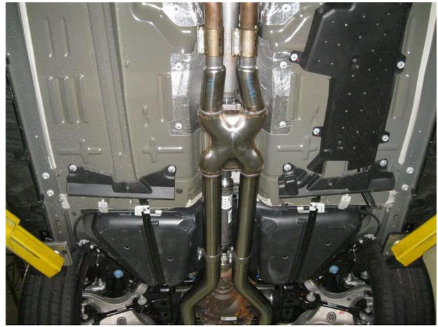
**Step 3.** Begin installation of the new system by loosely attaching the X-Pipe Assembly to the outlets using the OEM clamps. Leave all clamps loose until final adjustment.
