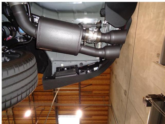
**Step 5.** Finish the initial installation by fitting the Muffler Assemblies onto the Mid pipe Assemblies using the supplied 3.00" clamps and inserting the hangers into the rubber insulators.
