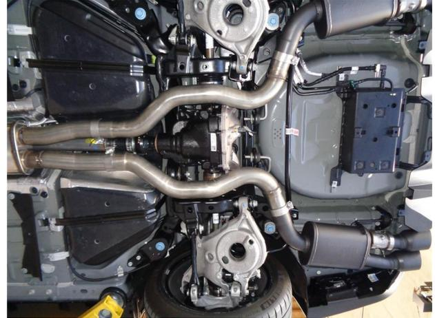
**Step 4.** Next attach the Mid Pipe Assemblies to the X-Pipe using the supplied 3.00" clamps and fitting the hangers into the rubber insulators.
