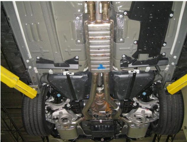
**Step 2.** Begin removing the OEM exhaust system by loosening the clamps located in front of the resonator. Next working front to rear extract the hangers from the rubber insulators and remove the OEM system. Retain insulators and clamps as they will be used to install the new system.
