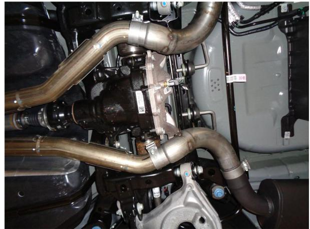
**Step 3.** Begin installation of the new system by attaching both Inlet Pipe Assemblies to the pipes you have just cut. Loosely secure using the supplied 2.50" clamps. Engage the welded hangers to the rubber insulators. Leave all clamps loose until final adjustment. If equipped with valves, be sure to reinstall valves on new system with wire harness mounting bracket.
