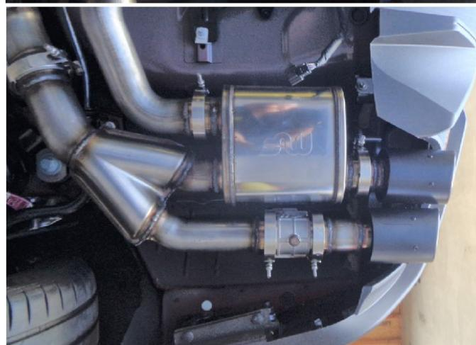
**Step 6. The NDT Muffler assemblies are shipped with the xTreme Bypass modules installed without the xTreme Bypass Block-Off Plates. Depending on preference, there are four different exhaust configurations possible with this system in either non-Active Exhaust (See Page 5) or Active Exhaust configurations (See Page 6).**
