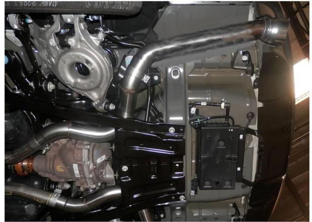
**Step 3.** Next attach both Tailpipe Assemblies to the Inlet Pipe Assemblies using the supplied 3.00" clamps and fitting the hangers into the rubber insulators.
