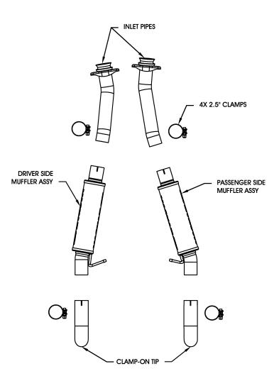
NOTE: Magnaflow Performance exhaust systems are designed for a correct fit on vehicles with OEM components. Aftermarket accessories such as headers, and/or cors-over assemblies (H-pipe /X-Pipe) may not fit like the OEM components, and may require fabrication for proper fit of your MAGNAFLOW system.
