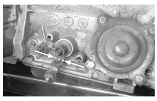
**28.** Move the selector lever to NEUTRAL (2 clicks from PARK). If the selector lever points downward, cut it off at the inboard bend, to allow correct positioning of the B&M lever.
