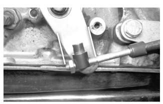
**32.** Thread the swivel onto the cable to about the middle of the threaded section, then reinstall (but do not yet tighten) the jam nut.
