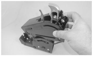
57. Install the cover. Verify the shifter mechanism is free of any debris or loose hardware. Remove the two screws from the left grip plate, carefully move the plate behind the grip, and lower the cover over the shifter. Then secure the cover to the shifter with the two quick-release pins, and reinstall the grip plate.
