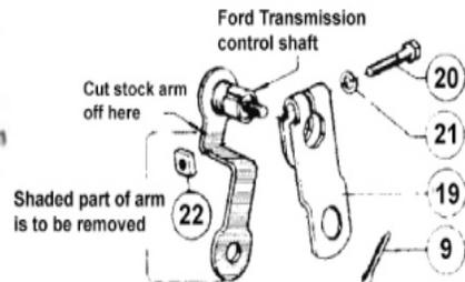
Cut shaded part of stock arm off. Install Hurst arm on shaft loosely using the supplied hardware. Do not tighten at this time. Follow the adjustment procedure outlined in the body of the instruction sheet.
