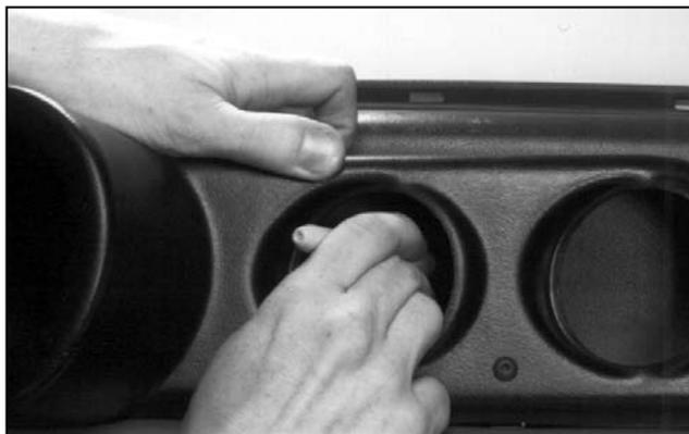
5. Remove bracket screws and pod.
