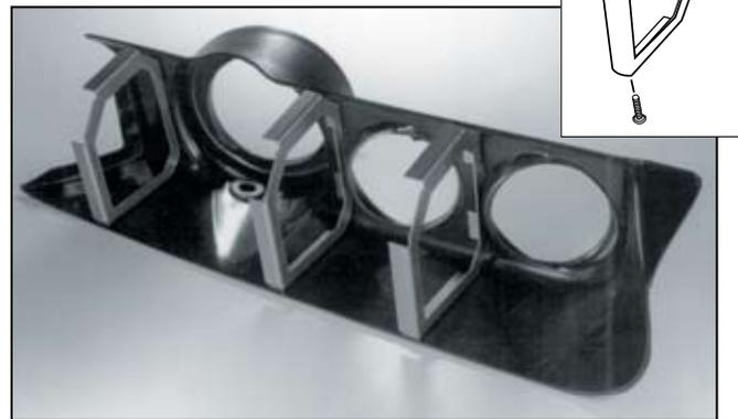
3. Place Tach Pod on dash. Apply pressure on top front edge of pod to settle it in position. Due to slight variations in dashes the Tach Pod may need to be trimmed for a perfect fit.
