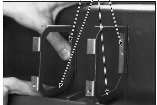
8. 2<sup>5</sup>/<sub>8</sub>" gauges require mounting brackets to hold them in place (see gauge instructions for mounting). Tach mounting is a press fit. If a shift light is used, follow instructions below.
