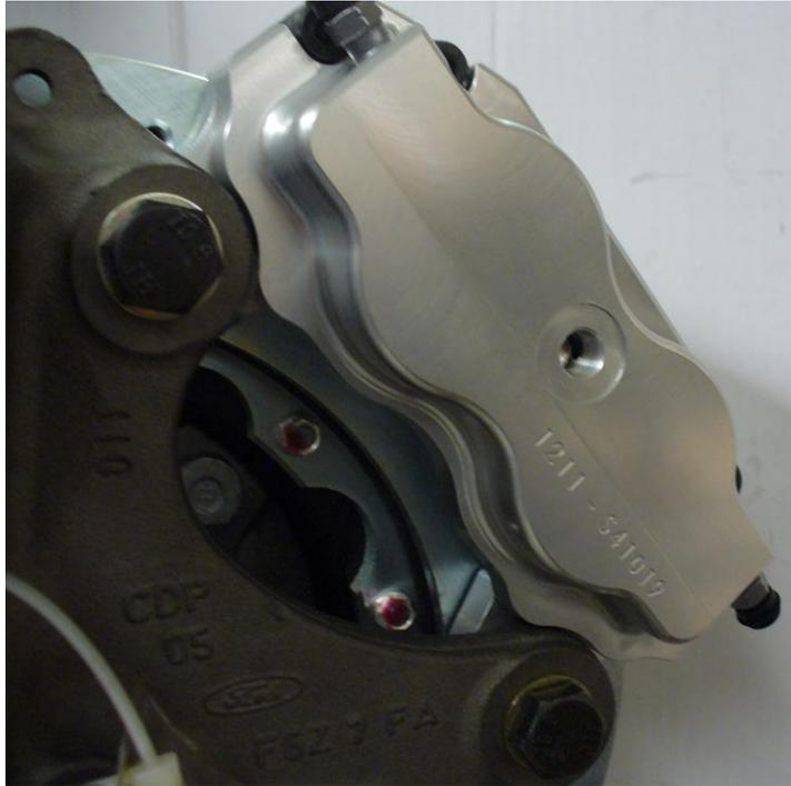
\*\* Note: All or most S4 Calipers are made with dual bleeders for orientation depending on the setup.
