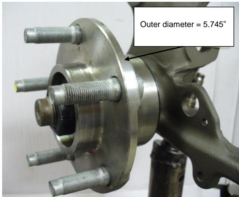
4. If needed, reinstall the hub back onto the spindle, ensuring that the spindle is clean and free from any damage. Carefully slide the correct side rotor on the hub and secure it with one lug nut and one washer. This will prevent scratching of the rotor hat.
