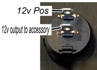
**On/Off Switch Wiring**
