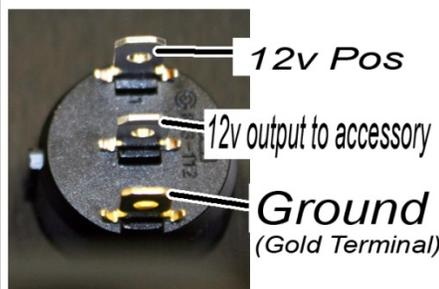
**Bottle Opener Switch Wiring**
