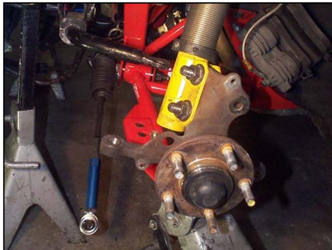
102. Attach the adjustable outer tie-rod end to the spindle. As a starting point, place a 2" stack-up of spacers between the spindle and the tie-rod end. Torque the tie-rod end bolt to the specification stated in your adjustable tie-rod end kit.
