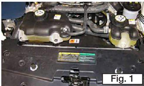
2. Remove the coolant tank cap from the heat exchanger coolant tank.
