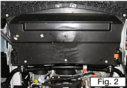
6. Remove the 10 clips from the fender well splash guards. Pull the splashguards back from the front bumper and remove completely.
