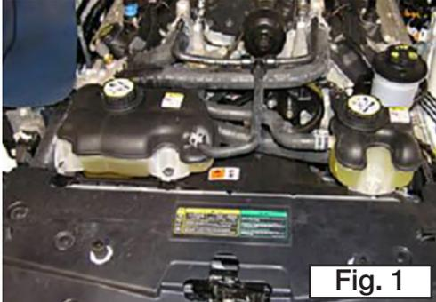
2. Remove the coolant tank cap from the heat exchanger coolant tank.
