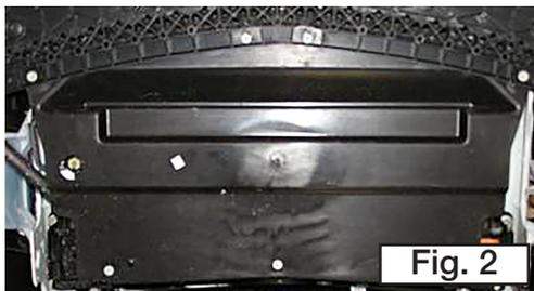
6. Remove the 10 screws and clips from the fender well splash guards. Pull the splash guards back from the front bumper and remove completely.
