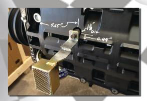
Image left shows the location you will need to modify the tray in order to properly mount the pickup tube. In addition to this modification you will also need to move the pickup mounting bolt from the OE position to this location.
