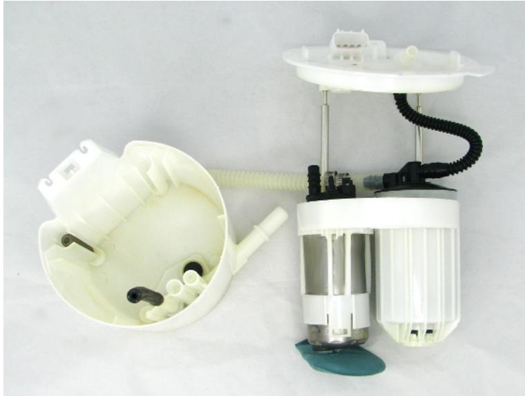
6 – install assembly center section into the assembly bucket and connect the 3/8" tube to the outlet of the pump, then pinch the 13.3mm permanent clamps. Slide the larger permanent clamp (7mm) onto the hose and crimp it in place (over the barbs) with a pair of side-cutters. Slide the smaller permanent clamp (6.1mm) on the hose and install the free end on the smaller venturi outlet on the pump. Crimp the clamp in place under the barb
