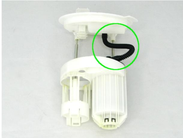
4 – remove the 3 locating tabs and smooth the pump receptacle to the diameter of the DW400 (46mm)
