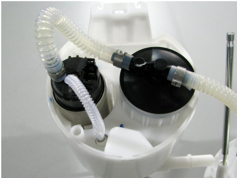
7 – install the supplied DW connector harness, the additional static ground inserts into the slot on the assembly filter, the same as OE
