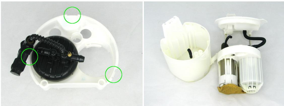
3 – carefully cut the larger pump outlet tube (3/8" ID) from the assembly filter and remove the OE pump, the supplied DW 3/8" ID tube will be used later. DO NOT cut the 3/8" ID tube that connects the assembly filter to the assembly top-hat (circled in green)
