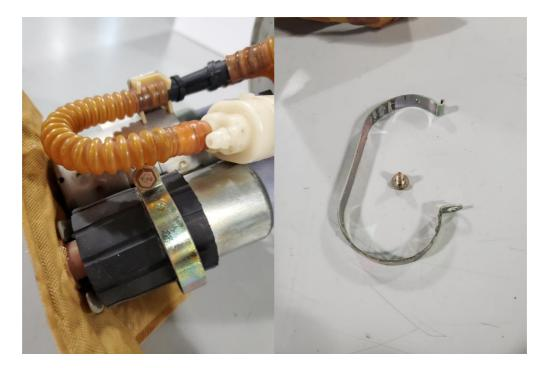
2 – Unplug the factory electrical connectors, it may be easier to use a small flat head screwdriver or a pick tool to depress the latch due to the crowded nature of the module.
