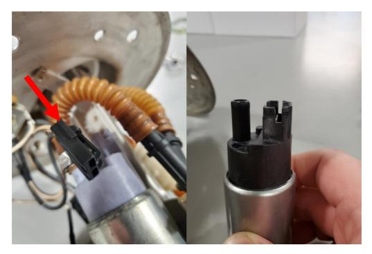
4 – Remove the factory convoluted tubes from the top of the Y-Fitting. This is typically done with a knife, take care not to damage the fitting under the tubing. Once loose remove the pumps from the module.
