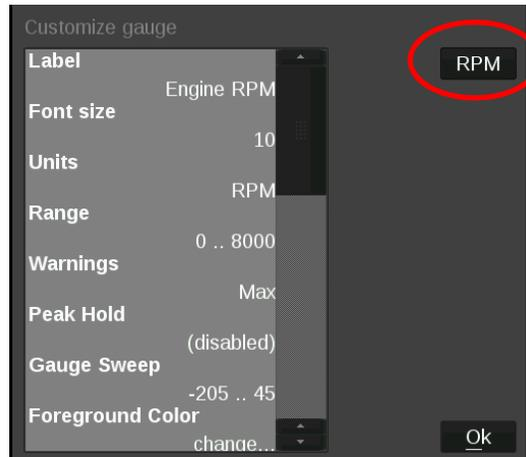
**NOTE: Only the gauge value being displayed will be updated, the user MUST manually change Labels, Units, Range, Warnings, etc. with proper values as these will NOT be updated automatically! Refer to the ‘Customizing Your Layout’ Section of this manual for instructions on gauge customization.**
