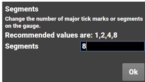
**NOTE:** Ensure the number of segments is matched up with the range you specify. E.g. If you choose 6 segments in a 0-8000 tachometer range, the scale markers will be at 0, 1333, 2667, 4000, 5333, 6667, and 8000. For this example, we would recommend using 4 or 8 segments instead.
