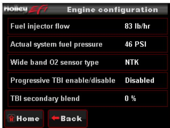
**Fuel Injector Flow:** Adjust fuel flow injector ratings to match what is installed on the engine
