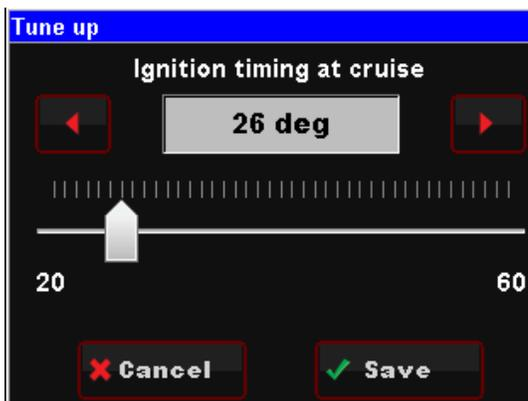
All Holley base tunes contain timing curves that will provide adequate engine operation, however the ignition timing at idle, cruise, and wide open throttle can be adjusted independently from each other to compensate for geographical and climate extremes.
