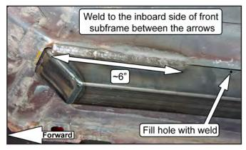
31. The two Middle Side Plates of the subframe connector tube will need to be custom-fitted into place against each side of the car's front subframe. This can be done by squeezing them with a C-clamp or large channel lock pliers, or by careful hammering. We position the plates to accommodate the range of tolerances in the placement of the front subframe on the floor pan, which requires the plates to be custom-fitted to the car during installation.
