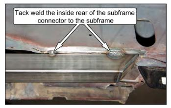
29. Weld the rearward end of the subframe connector into place. Weld where indicated in the photos.
