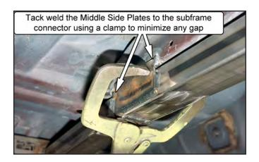
32. Weld the two Middle Side Plates to the car's front subframe, as indicated in the photos.
