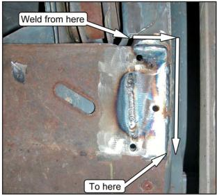
9. Weld through the slits made in Step 7 to the factory subframe.
