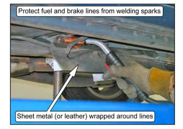
26. Tack-weld the four legs of the seat brace to the subframe connector.
