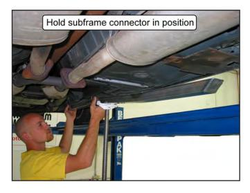
NOTE: The connectors fit specific sides. The forward end of the subframe connector tube has a Side Plate, which is to be positioned on the outside of the front subframe.
