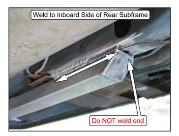
30. Weld the forward end of the subframe connector into place. Weld where indicated in the photos. Do not weld across the end-cap, as doing so will create a heat-affected zone on the subframe that may later lead to cracking due to the orientation of the weld relative to the bending loads. The holes through the side of the tube must be filled in with tack welds to prevent rust.
