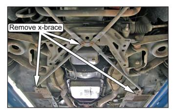
3. Using a drill bit or die grinder, remove the rivets retaining each of the front factory reinforcement plates to the vehicle.
