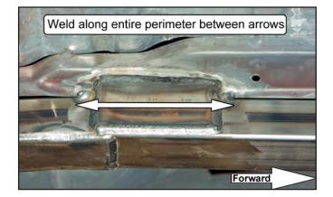
33. Weld the legs of the seat braces to the subframe connector. Make sure to wrap the welds around the ends of the legs.
