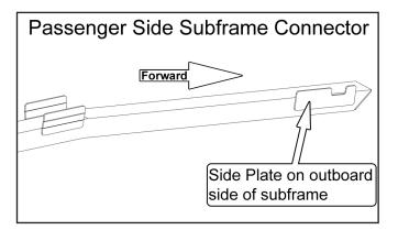
14. Place a straightedge on the front subframe connector end-cap, extending above the top surface of the connector by about 1". Use the straightedge to align the front of the subframe connector with the car's front subframe, where the front subframe angles upwards. This sets the fore and aft position of the subframe connector. Mark a line along the forward edge of the end cap to mark the correct position.
