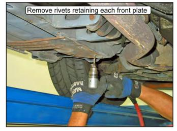
4. Remove the front factory reinforcement plates from the vehicle.
