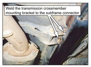
37. If so desired, the subframe connector tube may be stitch-welded to the car's front subframe. Weld the corners of the subframe connector tube to the car's front subframe. A 1-inch weld every 3 inches is sufficient.
