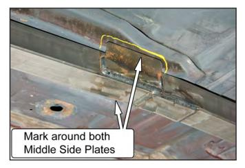
20. Remove any coating in the marked areas down to bare metal. A power disc sander works well for this.
