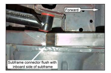
17. Check how closely the subframe connector fits to the underside of the car's *front* subframe. A gap of no more than 1/8" is acceptable.
