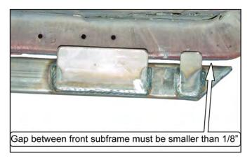
18. If there is a gap between the car's front subframe and the subframe connector at its front end, the subframe connector tube needs to have its forward bend straightened. Very small changes in the bend angle will have a large effect on the gap. The subframe connector tube can have the bend angle straightened out slightly while off the car by careful use of a hydraulic press. If using a press, be careful not to crush the tube.
