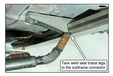
27. Tack-weld the forward end of the subframe connector in place.
