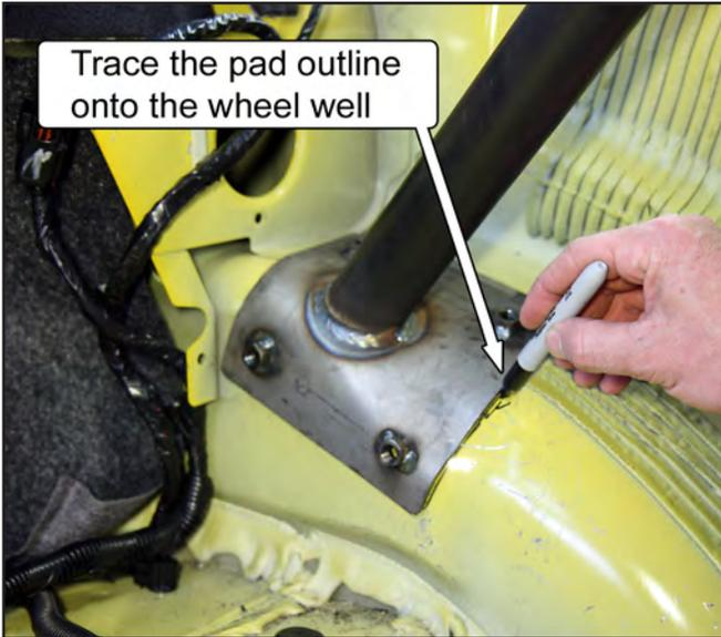
28. Remove the sound-deadening material within the outline using a chisel or other scraping device. Once done, reinstall the roll bar.
