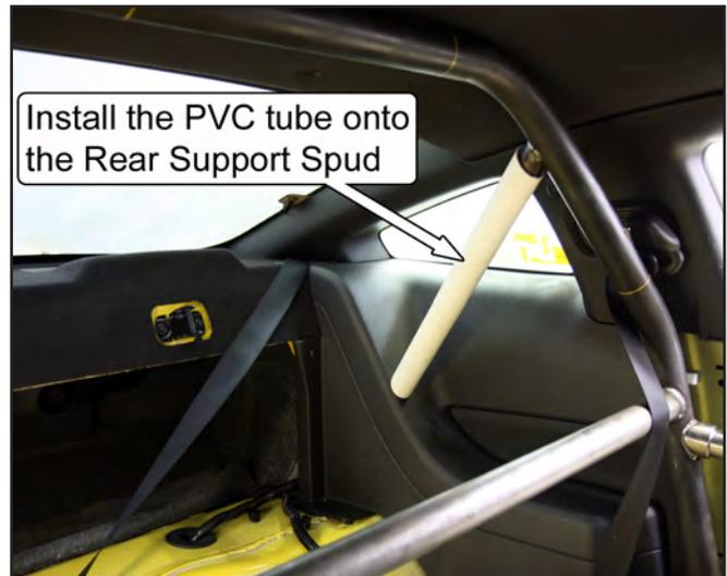
51. Set the roll bar back in its mounting position and slide the PVC template down until it contacts the plastic quarter panel. Rotate the PVC tube so the end is parallel to the face of the panel.
