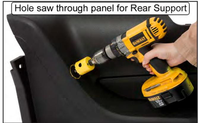
54. Cut a vertical line from the bottom of the plastic panel up to the rearward edge of the hole. This will allow you to slide the panel onto the rear support during installation. Use sandpaper or a file to remove any plastic burrs.
