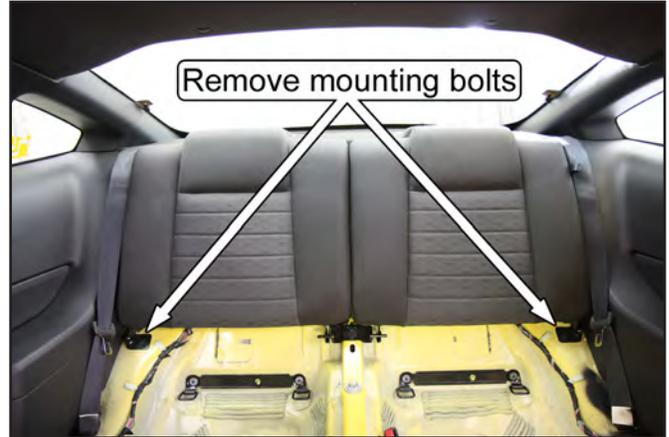
8. Pull the release strap to pivot the backrests down and slide the backrests off of the center pivot bracket to remove them from the car.
