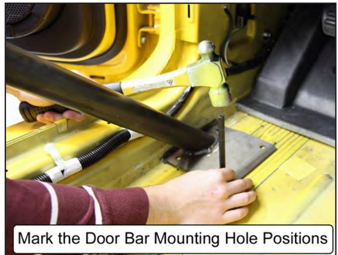
36. Remove the roll bar from the vehicle and drill the four holes marked on each wheel well out to a 7/16" diameter. Use a ~1/8"-diameter pilot drill to start the holes.
