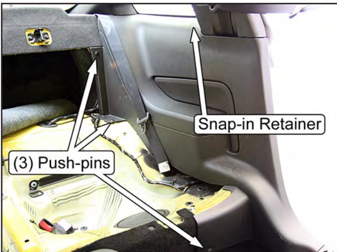
12. Remove both front plastic kick panels. Pull the portion closest to the firewall inboard to disengage the push-pin retainer, and then pull the panels rearward.
