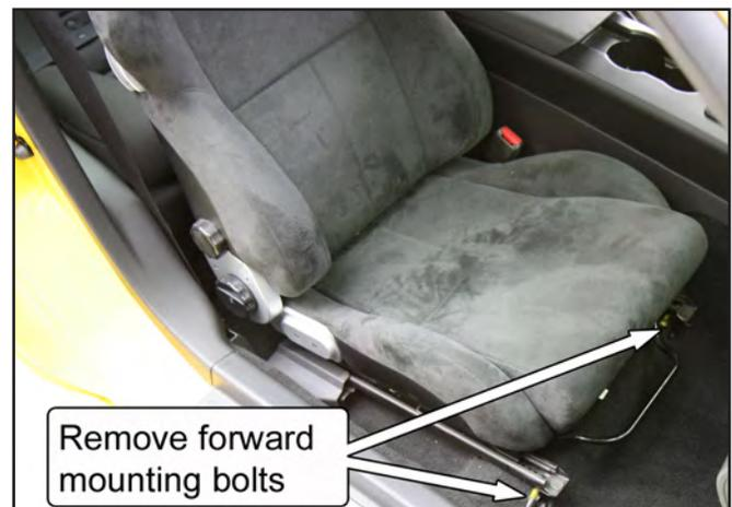
4. Tip the seat back to disconnect the wiring harness connectors for the air bag module and seat. Pull the seats out of the car and put aside.
