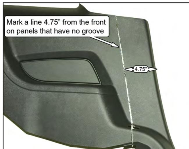
44. At the bottom of the quarter panel, extend the line across the horizontal flat. Add a mark about 3/8" forward of the line, centered side-to-side on the flat section.
