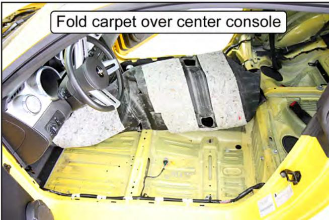
**NOTE:** If present, disconnect the wiring harness connected to the seat belt so the carpet can be folded over the center console.
