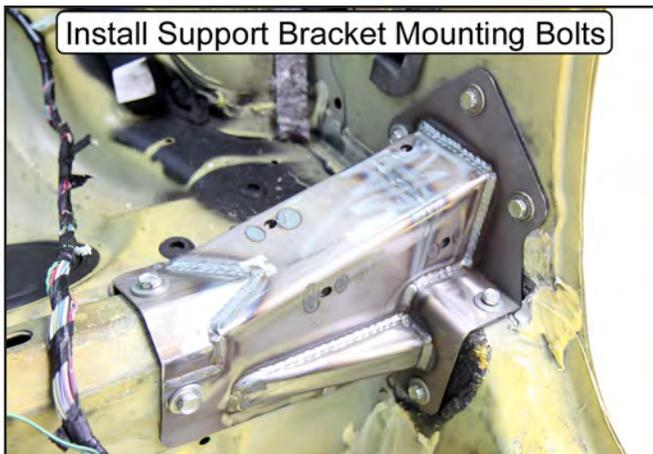
22. Using a wrench, tighten (but do not torque) all of the bolts in numerical order from H1 to H9 so the bracket can be properly seated against the vehicle.
