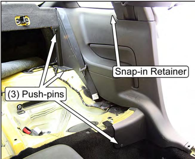
12. (DB ONLY) Remove both front plastic kick panels. Pull the portion closest to the firewall inboard to disengage the push-pin retainer, and then pull the panels rearward.
