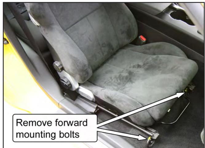
4. Tip the seat back to disconnect the wiring harness connectors for the air bag module and seat. Carefully pull the seats out of the car and place aside.
