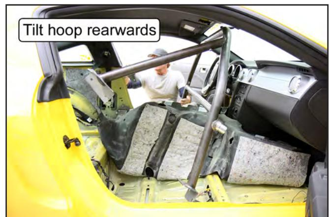
27. Trace an outline of the rear support mounting pads onto the driver- and passenger-side wheel well, and then remove the roll bar from the vehicle.
