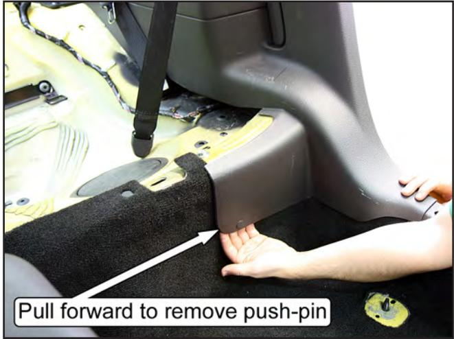
11. Remove the rear quarter panels. There are three push-pin retainers on each panel; one is located at the front of the seat bulkhead and two are at the rear seat backrest. Carefully pull the rear half of the panels inward to disengage the snap-in retainers located below the quarter window, and then pull the panels forward.
