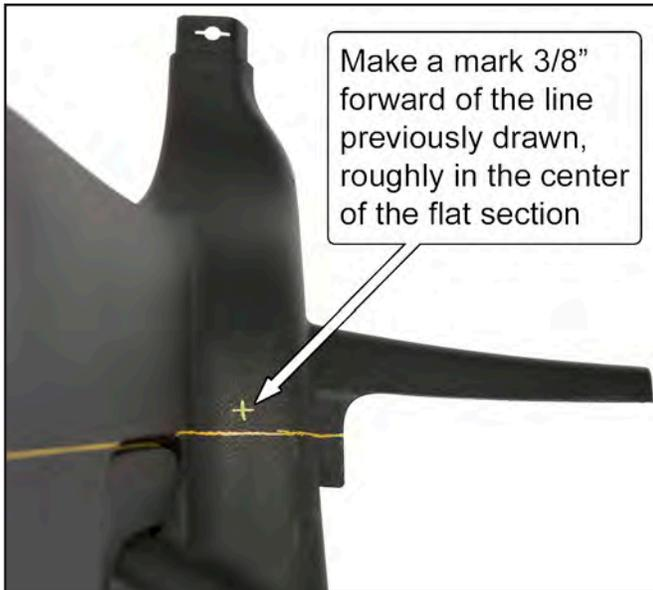
45. Using a 1-3/4" hole saw, cut a hole in the center of the flat, 3/8" forward of the marked line.
