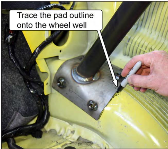
28. Remove the sound-deadening material within the outline using a chisel or other scraping device. Once done, reinstall the roll bar into the vehicle.
