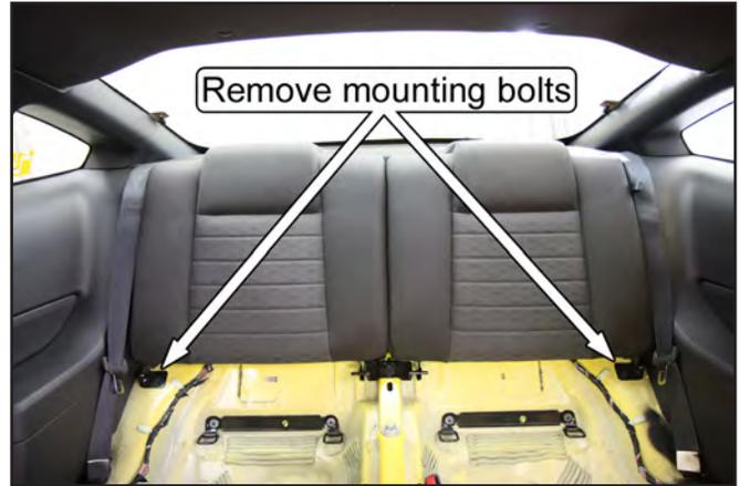
8. Pull the release strap to pivot the backrests down and slide the backrests off the center pivot bracket to remove them from the car.
