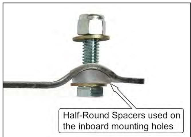
87. (DB ONLY) Torque the entire door bar mounting hardware to 33 lb-ft.
