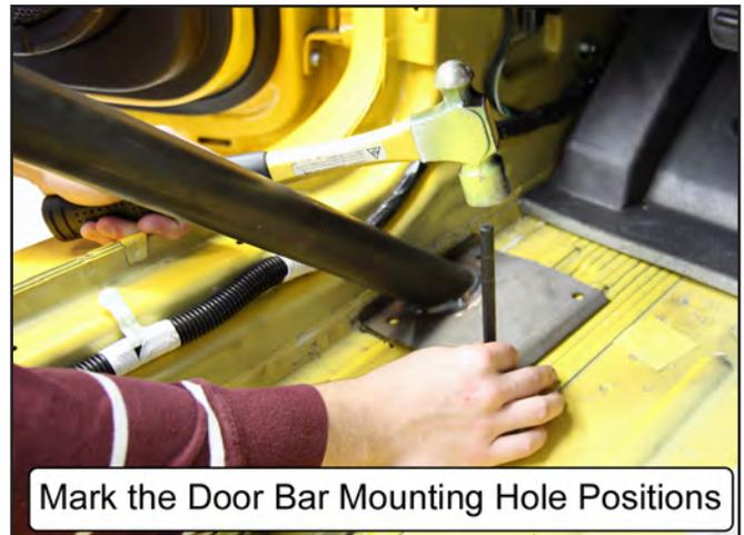
36. Remove the roll bar from the vehicle and drill the four holes marked on each wheel well out to a 7/16" diameter. Use ~1/8"-diameter pilot drill to start the holes.
