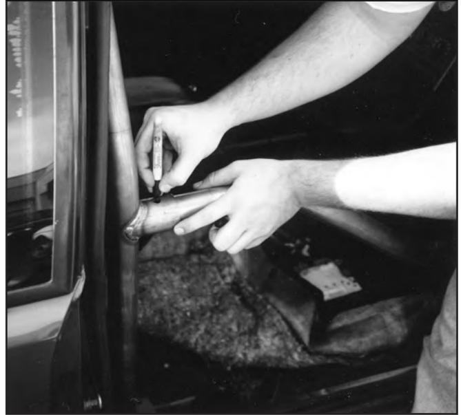
29. Place the door bars into position and insert the two 1/2" bolts at the main hoop.
