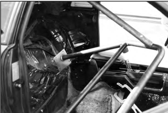
11. Tilt the main hoop upward and rearward to clear the steering wheel.
