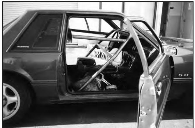
10. Move the driver-side mounting pads into the left rear seat area as you swing the passenger-side of the hoop into the car.
