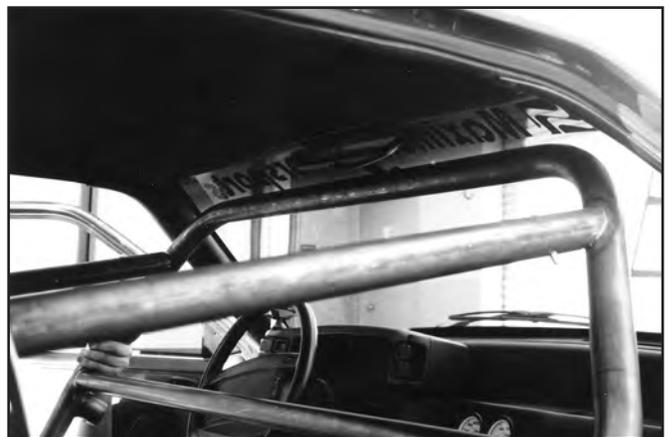
12. Pull the main hoop forward so the mounting pads are about 8–10" forward of the rear seat bulkhead.
