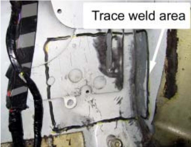
22. Using a power sander, carefully sand away any paint within 1/2" on either side of the outline made in the previous step. The paint must be fully removed to allow proper welding of the Weld-on Reinforcement Plate to the vehicle.
