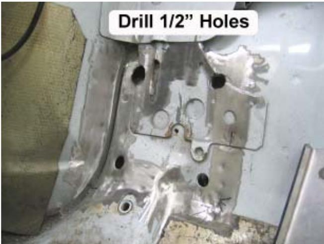
26. Reposition the driver side Weld-on Reinforcement Plate so that four pre-welded nuts on the backside of the Plate are centered over the 1/2" drilled holes. The top half of the pad should be resting flush with the floor pan and touching the inner fender well.
