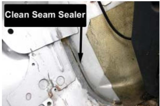
20. The Weld-on Reinforcement Plates are located in the vehicle as shown in the photo below. The stock floor pan area where the Plates will be located has two raised features that prevent the Plates from sitting flat on the floor pan. It is necessary to remove these raised features for proper installation. Using a grinding wheel, grind the raised features flush with the surrounding floor pan.
