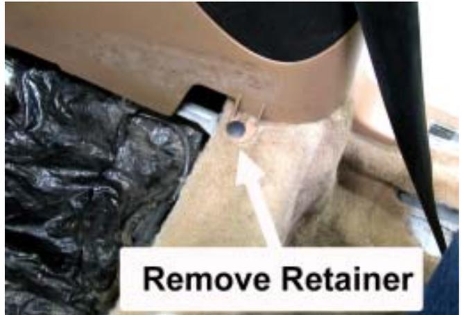
11. Remove the two small plastic retainers that are located on the forward face of the driver and passenger rear plastic side panels. Take care to avoid damage to the rubber door seal flap.
