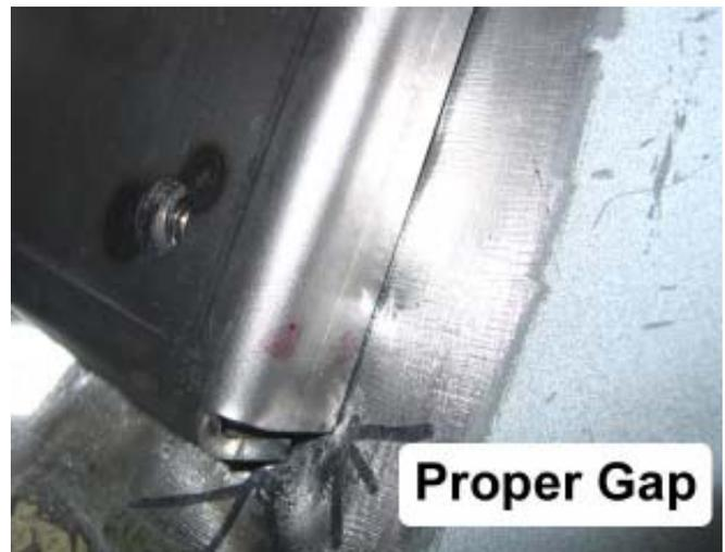
NOTE: On some vehicles the upper, outboard corner of the Weld-on Reinforcement Plates will be spaced away from the floor pan. If this occurs, place a screwdriver through the adjacent 1/2" hole that was drilled in Step 25 and carefully pry the sheet metal upwards to minimize the gap.
