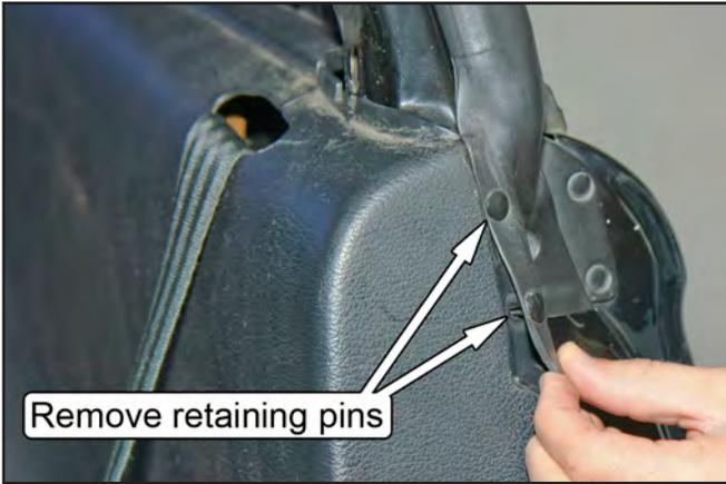
12. Remove the four retaining pins holding each lower plastic quarter panel in place. One pin is located beneath the quarter window, and the other three are behind the rear seat backs.
