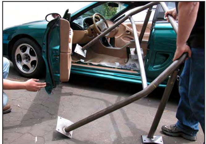
50. Again, have a helper hold the driver-side door open as wide as possible to avoid damage to the door.
