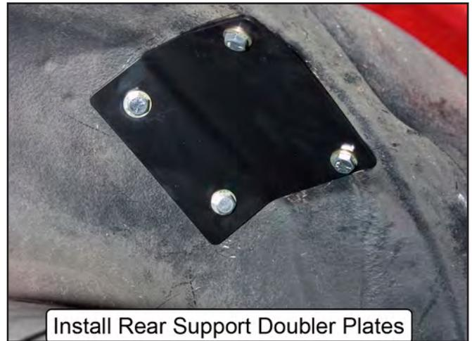
62. Install the main hoop doubler plates. Use 3/8"-16 x 1" long bolts, 3/8"-16 Nylock nuts, and 3/8" G8 washers beneath the bolt heads and nuts.
