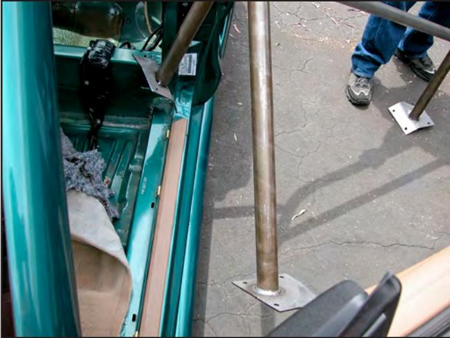
52. Make sure the rear support mounting pad clears the lower door frame and B-pillar, and complete the removal of the roll bar.
