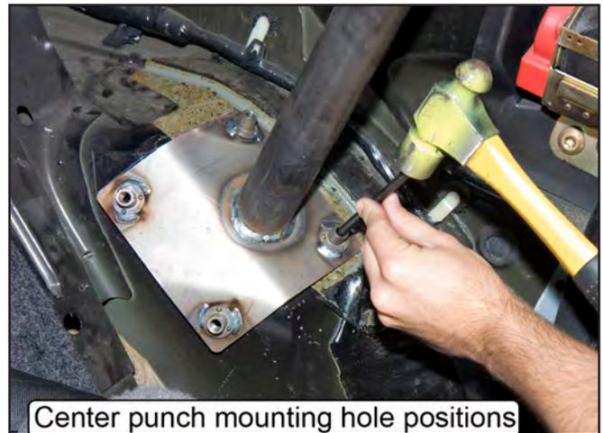
29. Move the main hoop forward and drill the four holes marked on each wheel well to a 7/16" diameter. Use 1/8" diameter pilot drill to start the holes.
