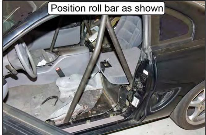
57. If desired, reinstall the sound insulation pads removed in Step 14. A couple strips of tape can be used to hold them up, off the wheel wells, until the roll bar is installed.
