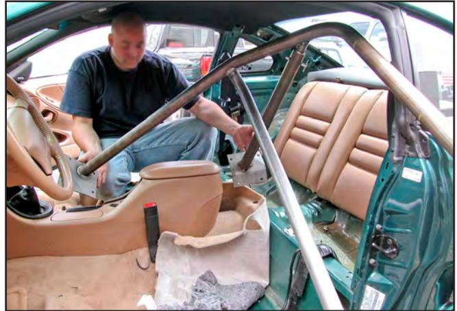
47. Keep the roll bar as low to the ground as possible in order to keep adequate clearance on the upper door frame.
