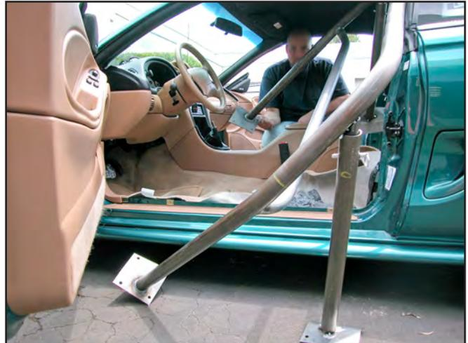
48. Pull the roll bar out the door and slightly toward the rear of the car.
