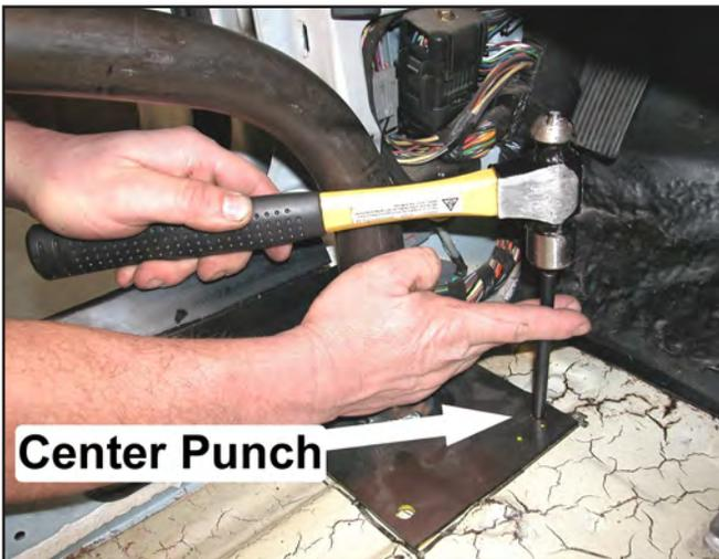
76. (DB Only) After removing the door bars, create a pilot hole at each of the center-punched marks using a 1/8" or similar-sized drill bit.
