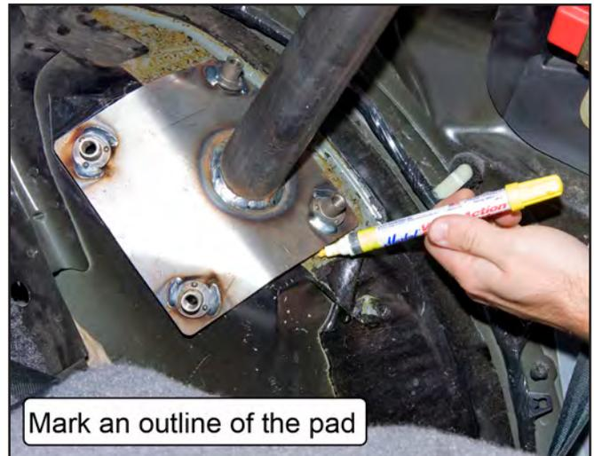
24. Move the main hoop forward and chisel away the sound insulation within the marked area on each rear wheel well. The rear mounting plates must rest directly against the metal of the wheel well.
