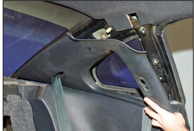
10. With the rear seats folded down, extend the rear seatbelts so that the panels can be placed in the trunk area, out of the way.
