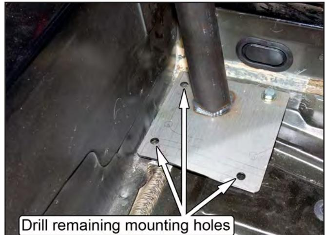
28. Mark the position of the four mounting holes in each rear support mounting pad onto the wheel well using a center punch.
