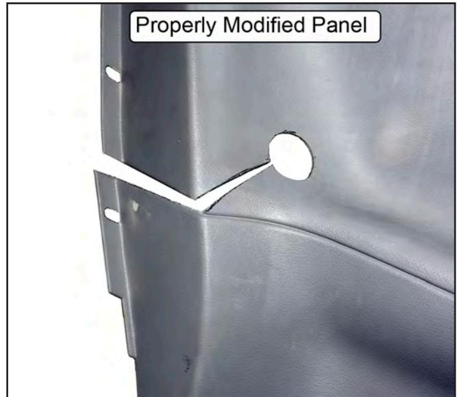
**NOTE:** 1994-98 vehicles use a less flexible plastic for the quarter panels that can't be spread apart. They require removal of a section of the panel to allow installation onto the rear supports. Remove a section of the panels **as shown below**.
