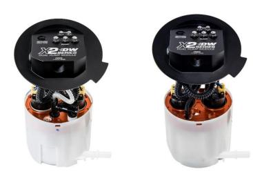
The new DeatschWerks X2-Series Mustang Module is now available for the 2011-2019 model years, which includes accommodation for 2 pumps (39mm or 46mm diameter pumps– your choice), integration of a return fuel line, and retention of ALL the functionality of OE module. The DW X2-Series Mustang Module consists of a top-hat, center section, and OE lower bucket. These 3 components work together to deliver the flow you need and the OE functionality you want.
