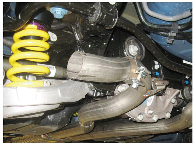
3. Insert the Roush muffler hanger into the mount at the rear of the vehicle, and then slide the new pipe over the existing pipe.
