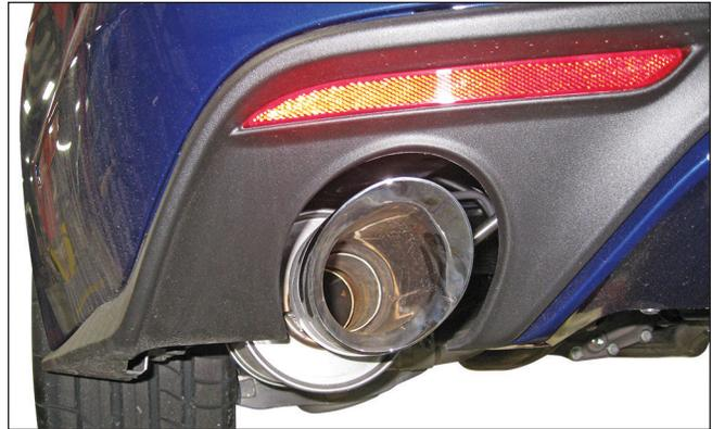
7. Once the desired position and alignment have been achieved, make sure all band clamps are torqued to 30 Nm.
