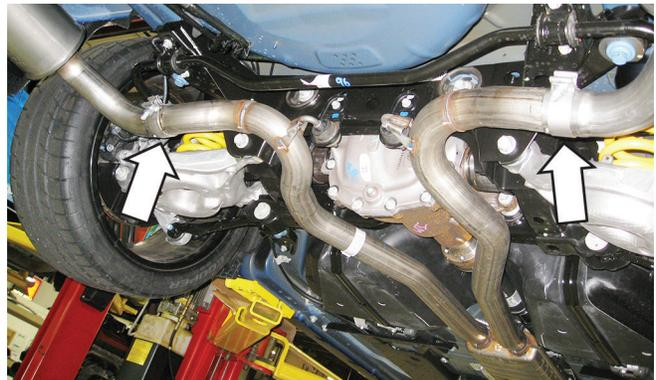
8. Before starting the vehicle, make sure to check all wires, hoses, brake lines, body parts, tires and any other components for safe clearance from the exhaust system.
