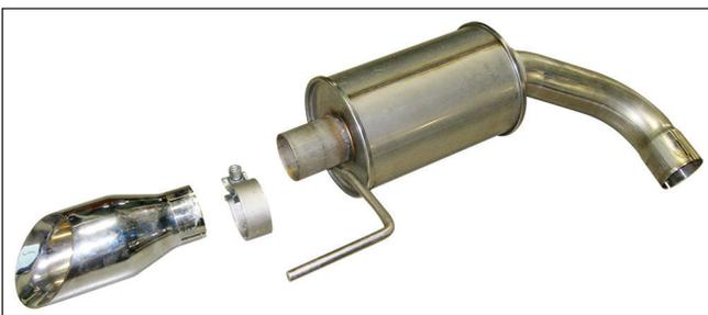
6. Check the exhaust system for correct clearance under the vehicle and also for tip alignment as shown below. If alignment is off, loosen the required band clamp, adjust, and re-torque the band clamp.
