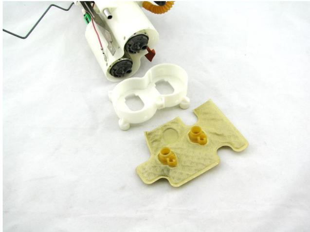
3 – disconnect the electrical connectors from the pumps and then pull the pumps out of the assembly
