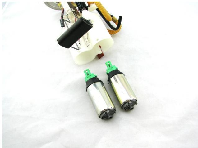
4 – the DW300m pumps are ready to install out of the packaging, install into the pump assembly and plug in the electrical connectors. The connectors on the original assembly should plug into the DW300m pumps. If the pump assembly has a different connector design than the DW300m or if the original connectors and wires are not in usable condition, wire in the supplied connectors from the DW kit
