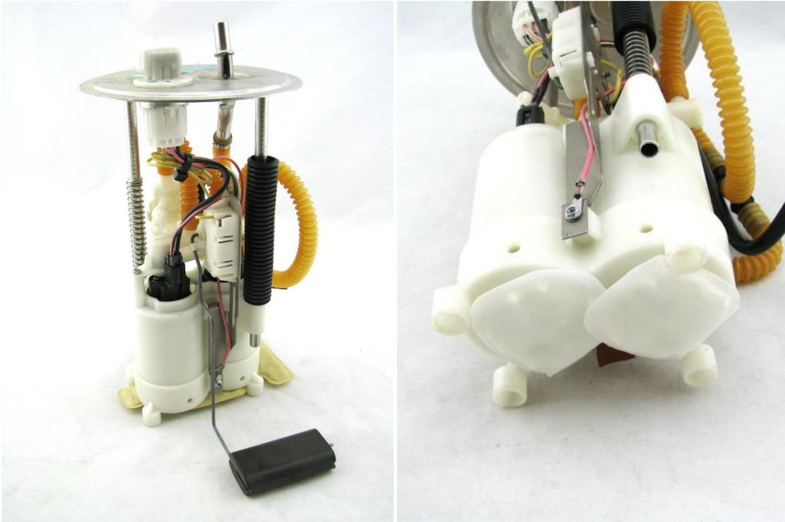
7 – reinstall the assembly into the fuel tank and attach a length of hose to the outlet of the pump assembly allowing it to drain into a fuel safe container and prime the fuel pump assembly
