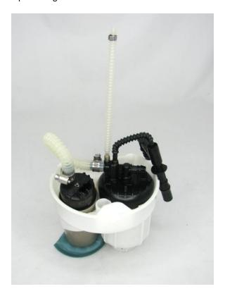
6 – install the center assembly into the bucket assembly and push the venturi manifold into the bucket assembly. Install the other end of the 1/8" hose to the bucket assembly and crimp the tang
