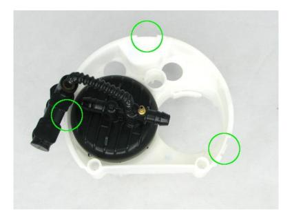
4 – carefully cut the pump holder out of the center assembly, be sure to leave some of the holder to give support for the DW400
