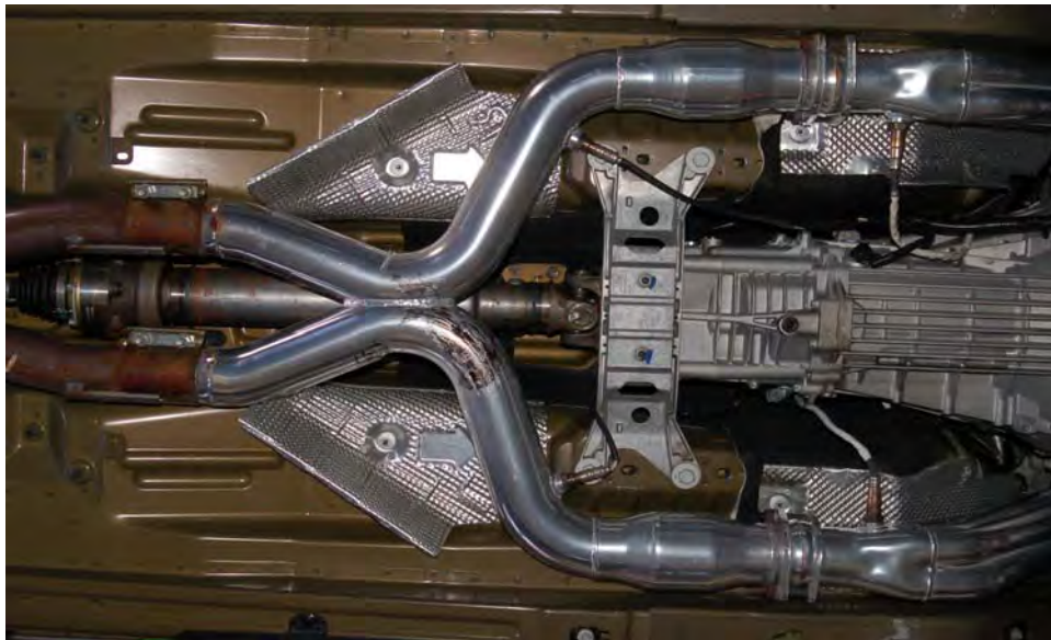
X-pipe shown installed Connects to stock rear barrel-style clamps
