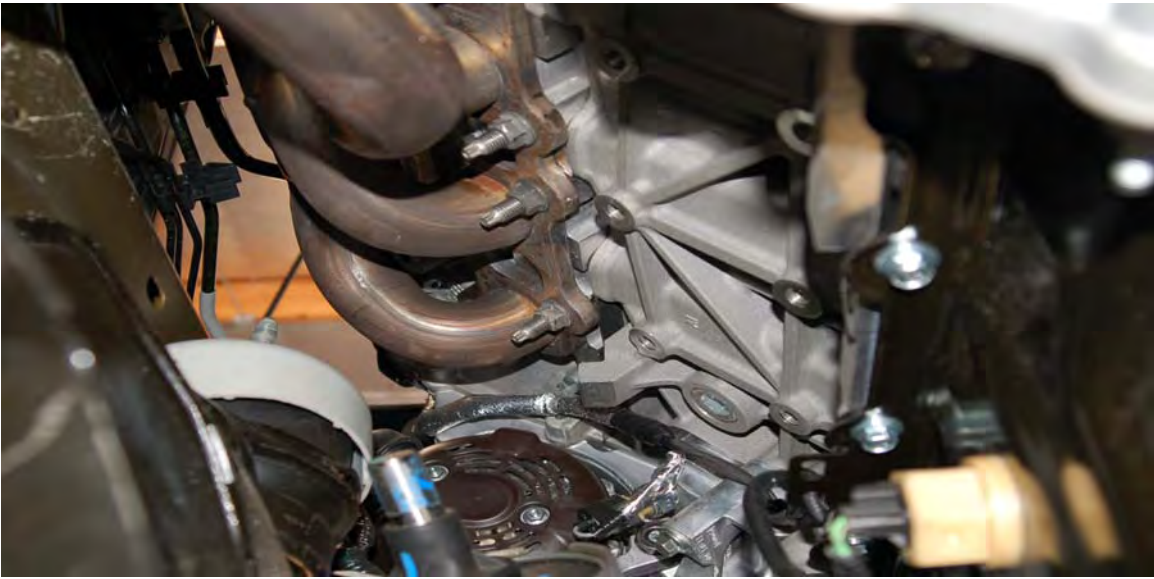
Fig 1. Motor Mount removed. Shows nut access.
