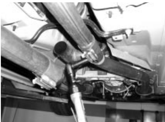
Separate H-pipe from tail pipe.
