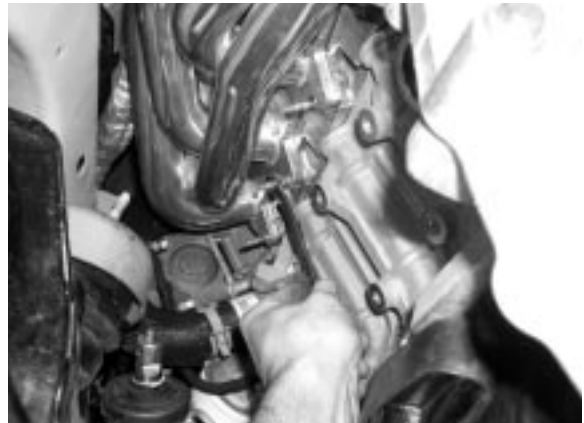
Remove dipstick tube.
