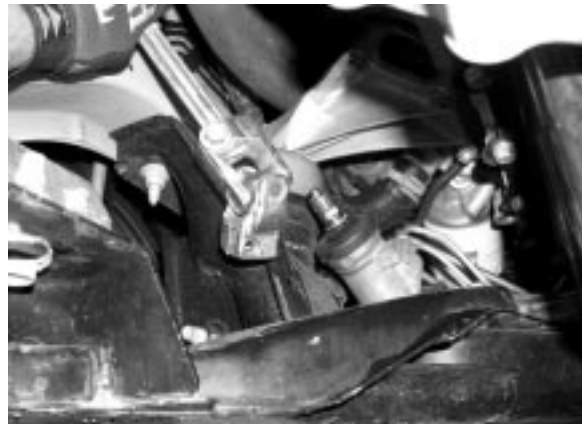
Disconnect steering shaft.
