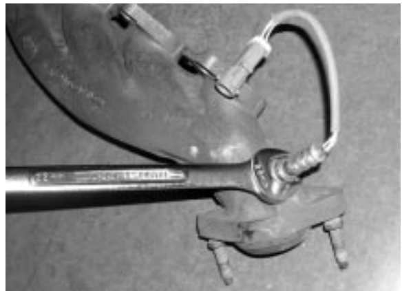
Removing the oxygen sensor.
